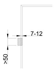
Installers must ensure that the resistance of the clamps is sufficient given the maximum pressure to which the module can be exposed. The clamps are not supplied by DualSun.
